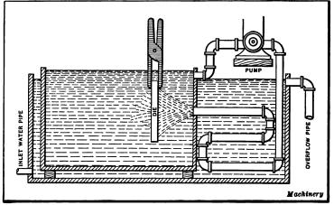
Fig. 27. Arrangement of Oil-cooling Bath for Dies
